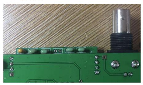
Now you have done the assembly of the TX portion. Before the TX test, please make sure the LPF band filter module and the band setting of Nano is matched. If not, please press and hold SW1-UP(BAND) button and power on so you can adjust. To adjust the band, you can press
