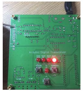
Press SW3-TX button to transmit, the nearby receiver will hear a quite strong signal. It is S9 plus 60dB on my TS-590 transceiver. I tuned to 14.074MHz because I have identified from the LED that the band is 20m and mode is FT8.
