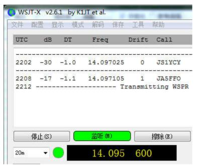
In main window, manually choose band the mode to display the correct working frequency. For example, if you choose WSPR and 20m band, the frequency will be 14.095600 and it is the same as the setting of the ADX-S firmware
