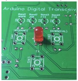
Populate D2-D5 and SW1-SW3 as close to the PCB as possible and solder.
