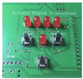
Now press and hold the SW2-DOWN(CAL) button and plug the power supply until you see both B1 and B4 LEDs are on. Now you can probe on the test point CAL using a frequency counter or other test instruments like an oscilloscope to see if you can get a 1MHz square wave. Please note,
