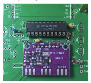
Now let's do a radiation TX test. Turn the board and power on. Use a probe of DVM to touch the center pin of Q3-BS170 as a radiation antenna.
