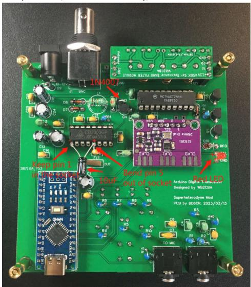
The red LED will reduce the amplitude of CLK2 (BFO) and also indicate the existence of CLK2 (BFO). The 10uF will enable AGC of CD2003. The 1N4007 in place of R13 is used as an attenuator in the RX front end.
