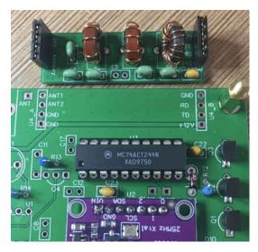
Plug the pin header sockets to the main board and solder.
