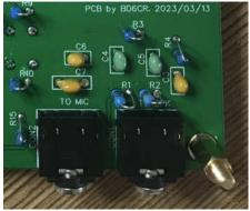
Use an audio signal generator like Sonic Tools App on iPhone to inject audio to CON1-TO SPK jack. Turn the volume to MAX and it should trigger TX, and the TX LED should be on. When you perform this test, please make sure the 50 ohm load is still connected to J1-BNC.
