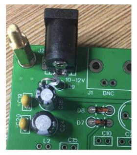
Now let's do a test to make sure the 12V does exist on VIN pin of XA1 – Arduino Nano module. Use the DVM for voltage measurement of about 12V. The red probe goes to the VIN pad, while the black probe goes to ground pad of the BNC connector. Plug in the 12V power supply (center positive) and measure. Looks good so far.
