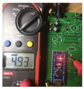
Measure 3.3V at the left pin of R1 - 1M. Looks good. Don't short circuit in this step, or the regulator will be damaged and it is very difficult to desolder the Nano module.
