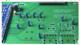
The long lead of the red LED goes to the + marking pad of D1.
